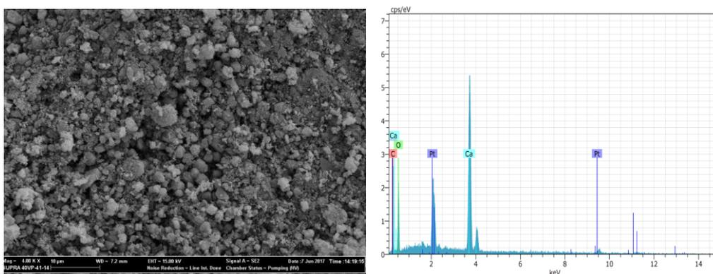
**Figure 2. SEM-EDS images of calcinated mussel shells**
