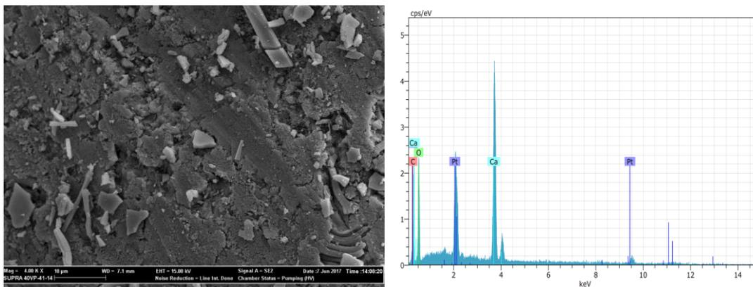
**Figure 1. SEM – EDS images of uncalcinated mussel shells**
